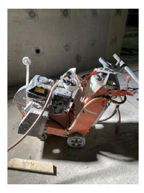
Figure 4-3 – Husqvarna FS400 LV Rotary Floor Saw.
