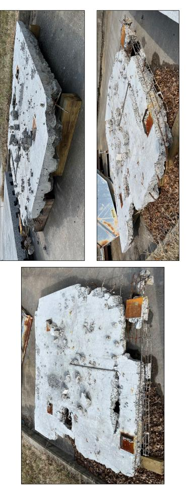
Figure 6.9.36: Images of the slab cut from the CF3 fire-tested floor. Orientation of the slab is unknown.
