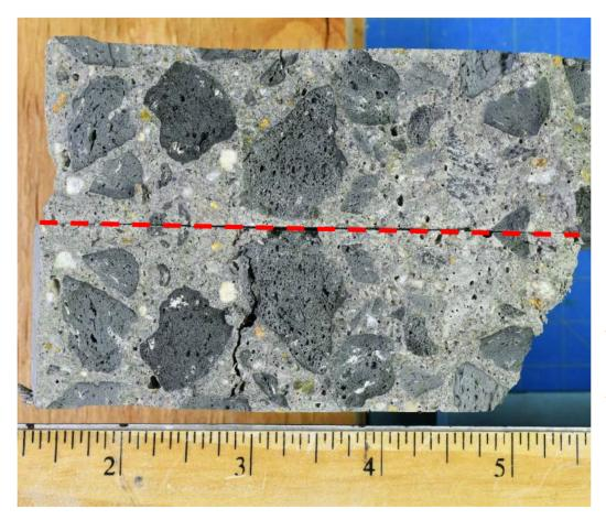
**Opposing surfaces** along a labcreated fracture plane on a section of Sample 4D-1. Most of the coarse aggregate particles are broken through along this fracture plane, which indicates a welldeveloped pasteto-aggregate bond. The red dashed line marks the division between the opposing surfaces.
