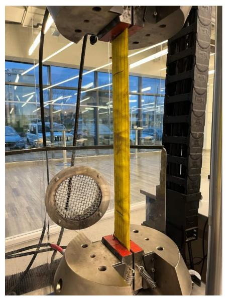
Photo 5-12 – Section of lifting sling used for tension testing in Instron machine
