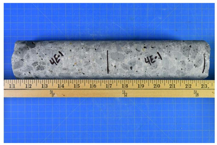
Photo 5-11 – Core extracted from sample 4E-1.
