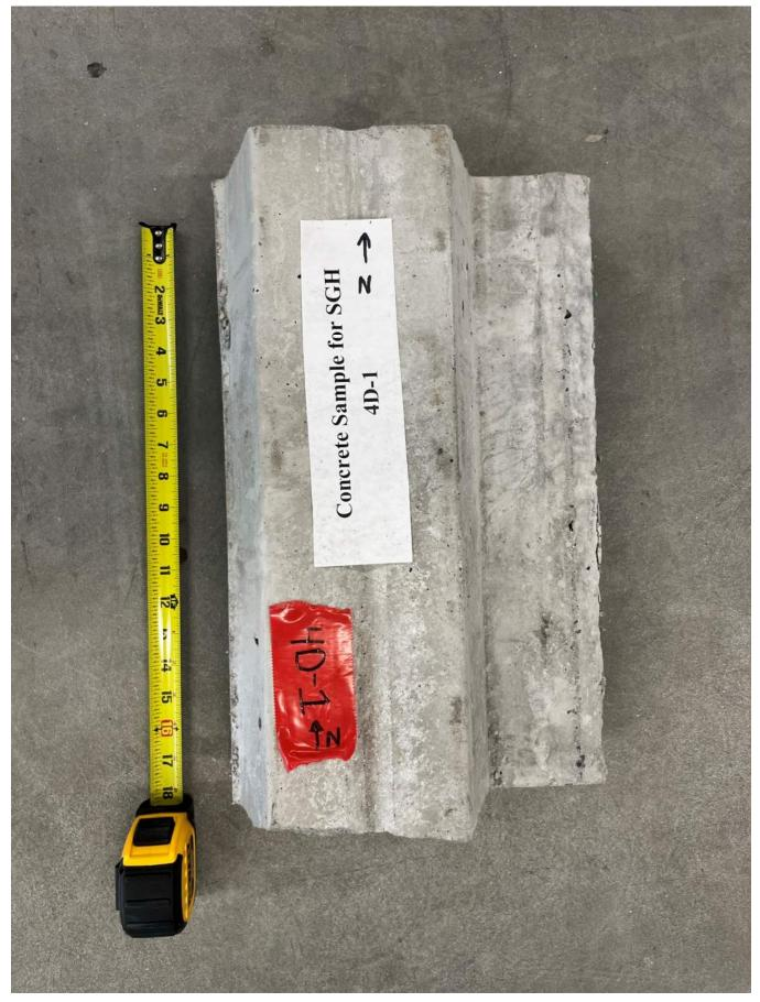
Photo 5-2 – Received slab sample 4D-1 (note direction indicated as North is actually South).
