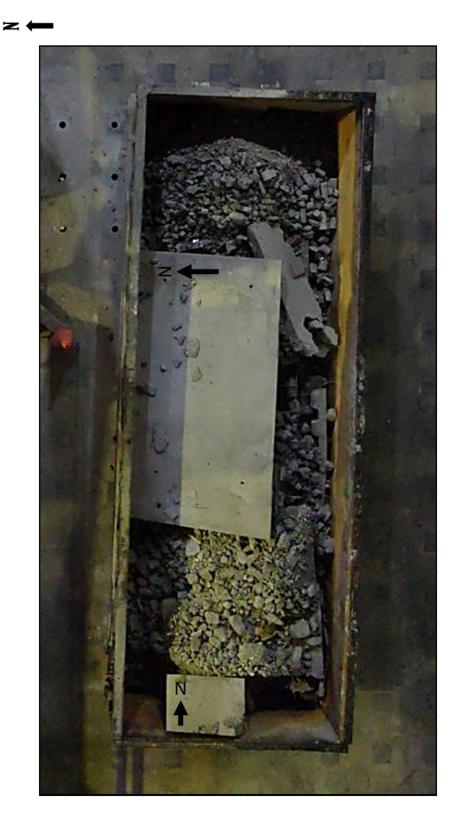
Figure 6.9.18: Image of both pieces of Slab 3. The northwest tab is rotated 90° clockwise in the roll-off and damage of the southeast corner can be seen from it having fallen to the strong floor.
