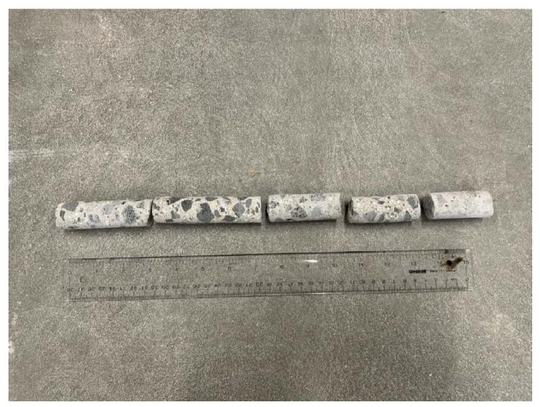
Photo 5-7 – Received concrete core sections.
