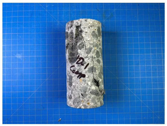
Photo 5-20 – Compression testing of specimen 4D-1 after peak load.
