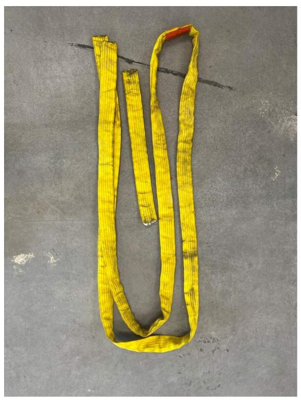
Photo 5-8 – Looped lifting sling with section removed for tensile stiffness testing.
