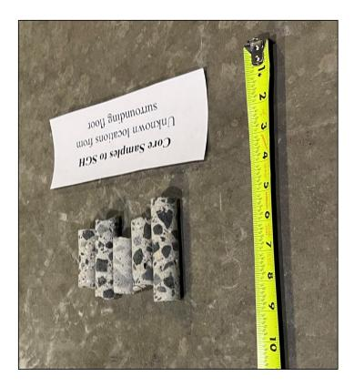
Figure 5.6.4: Core samples with 1 inch diameters from unknown locations in the surrounding floor sent to the contractor for analysis.
