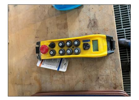
Figure 6.6.4: Crane remote used for the 20-ton overhead cranes in Room 125.
