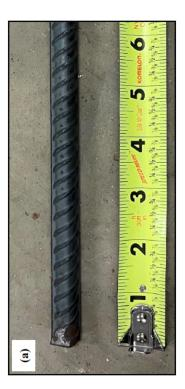
Figure 6.4.10: Images of steel reinforcement found in the concrete slab. (a) No. 4 rebar and (b) WWR mesh.
