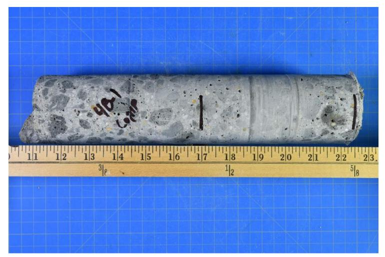
Photo 5-9 – Core extracted from sample 4B-1 with compression and tension halves identified.
