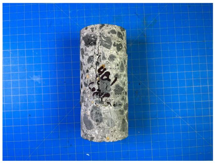
Photo 5-19 – Compression testing of specimen 4B-1 after peak load.
