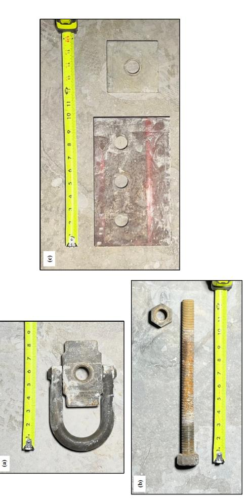
Figure 6.6.7: Images of the washers used as part of the rigging hardware. (a) Pivot lifting plate, (b) Threaded bolt with nuts, and (c) Two steel plates used as washers.
