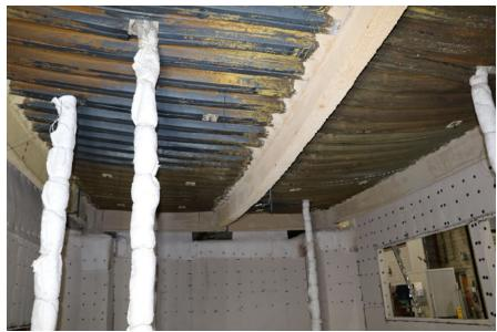
Figure 2-Bottom View of Damaged Test Section (Location of Shoring Installation)
