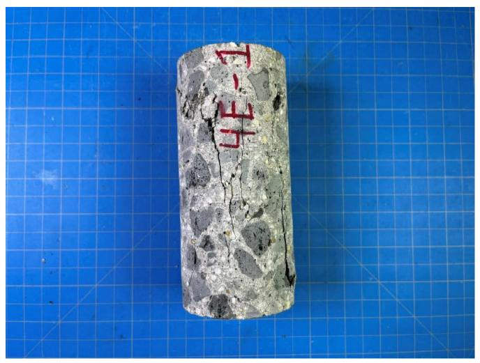
Photo 5-21 – Compression testing of specimen 4E-1 after peak load.
