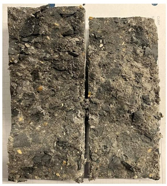
Photo 5-17 – Fracture surfaces of specimen 4D-1 after tension splitting.
