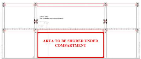
Figure 4-View of Shoring Area (Elevation View from South Looking North)
