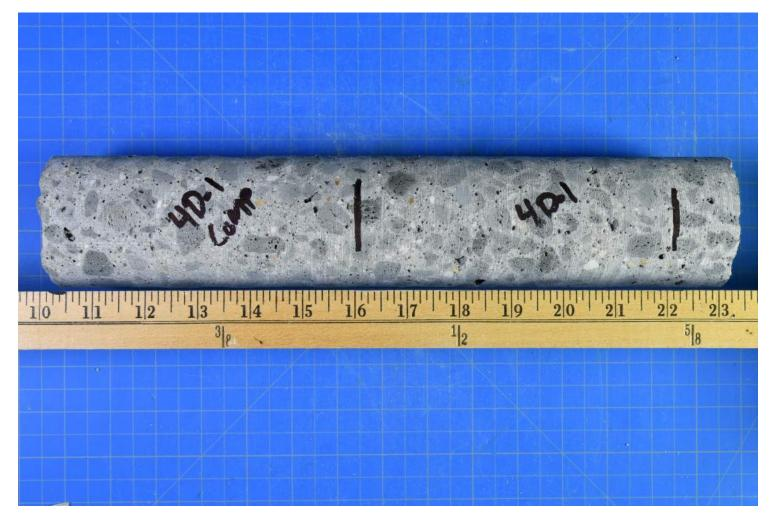
Photo 5-10 – Core extracted from sample 4D-1 with compression and tension halves identified.
