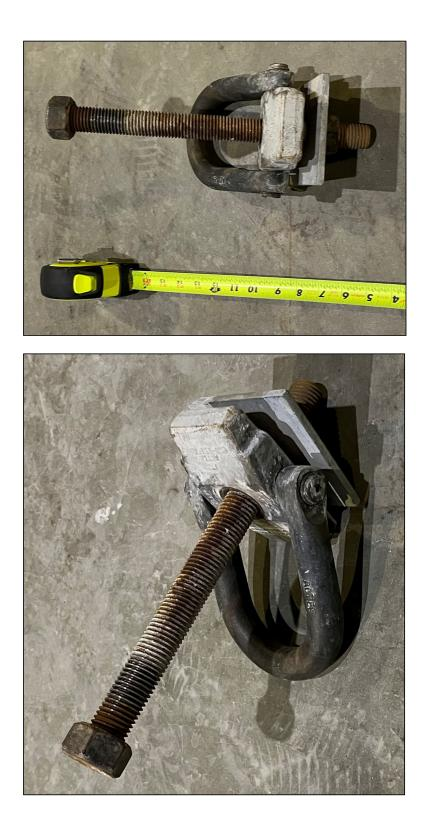
Figure 6.6.6: Rigging hardware assembly used to attach the rigging slings to the concrete slab. This specific set was attached to the northeast corner of Slab 4.
