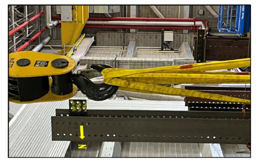
Figure 6.8.10: Post-incident image showing the overlapping of the slings on the crane hook.
