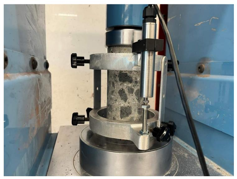
Photo 5-18 – Specimen 4D-1 with compressometer for elastic modulus testing.
